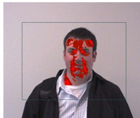
Figure 2. By using the color alarm feature, only the areas that exceed the 38 °C (100.4 °F) temperature threshold appear thermally.
