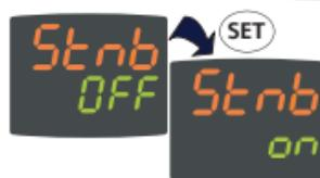
To change the status of a given function, press the **set** key.
