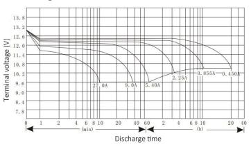
\* The above are average and date obtained from the first 3 charge/discharge cycles. These are not minimum values.
