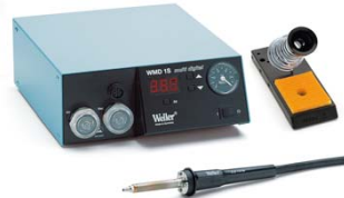
WMD 1A A single channel digitally controlled repair station with an integral pump to provide variable volume air flow and fixed value vacuum. The station is supplied with a 100 W hot air pencil but all other Temtronic tools of compatible rating could be driven.
