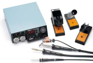
WMD 3K Three channel digitally controlled repair station with an integral pump to provide variable volume airflow and fixed value vacuum. The station is supplied with an 80 W miniature soldering iron, 80 W through hole desoldering tool and 100 W hot air pencil.
