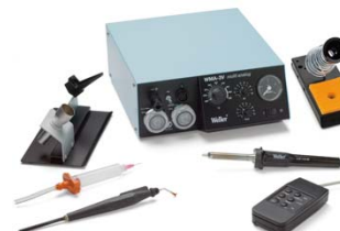
WMA 3V A single channel, analog controlled repair station for use with compressed air or inert gas. The station is supplied with a 100 W hot air pencil, vacuum pick up and solder paste/adhesive dispenser all able to be operated simultaneously.
