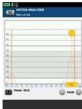
High Definition Time Domain Cross talk (HTDXTX) shows the far end connection is clearly the issue
