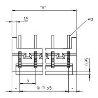
\*a solder pin for printed circuit board bore hole Ø 1.3 mm
