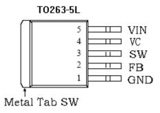
Figure 2. Pin Configuration of XL4015 (Top View)
