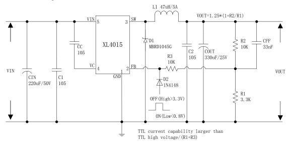
Figure 9. XL4015 Typical Application Circuit
