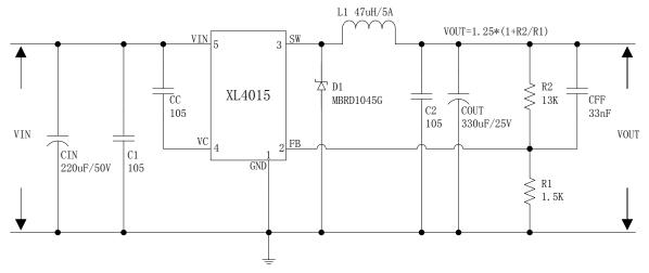
Figure 7. XL 4015 System Parameters Test Circuit (VIN=15V~36V, VOUT=12V/4A)
