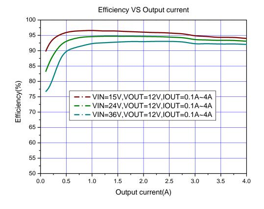
Figure 8. XL4015 System Efficiency Curve
