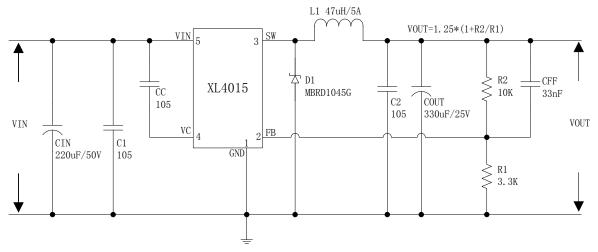
Figure 5. XL4015 System Parameters Test Circuit (VIN=8V~36V, VOUT=5V/5A)
