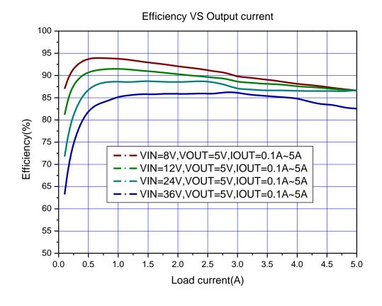
Figure 6. XL4015 System Efficiency Curve
