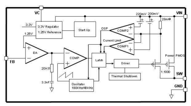
Figure 3. Function Block Diagram of XL4015
