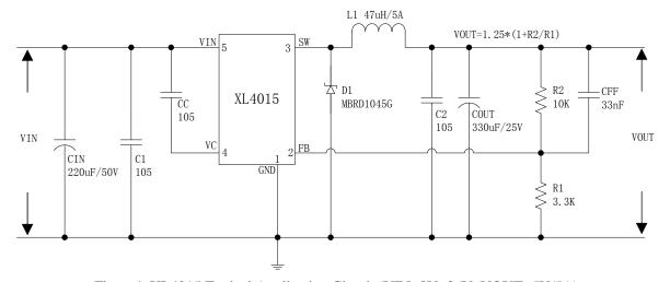
Figure 4. XL4015 Typical Application Circuit (VIN=8V~36V, VOUT=5V/5A)
