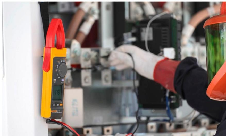
The Fluke 393 FC CAT III 1500 V Clamp Meter is useful for measuring dc power, ac/dc voltage and current, and for troubleshooting inverters.
