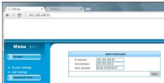
**Step 3:** Use a web browser to access the unit (TX:192.168.168.55, RX:192.168.168.56). Click the **System** menu and setup the required IP address, subnet mask, and MAC address as mentioned above. ***It is highly recommended to label the units with this setting. If you ever forget this setting you may have to reset the units to factory default values!***
