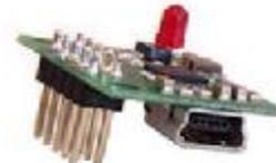
You can force the iSMART AS1 port to default communication with the MCBK36A operation by linking connector CN6 pins 3 & 4 on the iSMART module.
