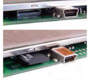
The SD Card can be connected to CN5 on the TFT using a suitable cable and adaptor.
