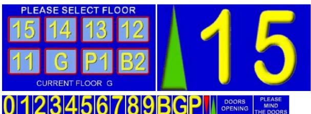
The user can select a floor and travel from any floor to another floor. The arrow is selected according to direction. Warning signs for doors opening and closing are used. Variables are used to store the current floor and destination floor. An RS232 interface could be added to communicate with other floor indicators. Download Image Files <zip>
