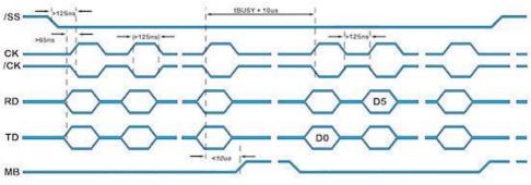
SPI Synchronous Serial Communication
