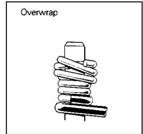
Keeping the tool on the terminal until the wrap is complete is important. If removed too soon, spiral and open wraps may result.
