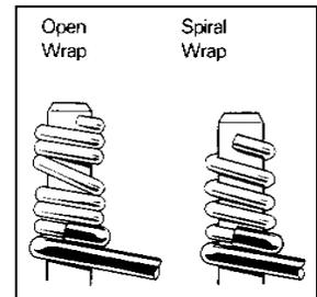
Feeding wire into the slot in the bit correctly is not difficult. The stripped end of the wire should be pushed in all the way.
