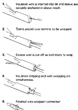
The cut-strip-wrap bit and sleeve assembly is an economical means for making solderless wrapped connections. The one-step operation results in time savings for terminating the loose ends of wire harnesses and cables when compatible combinations of wire and insulation tubes are used.
