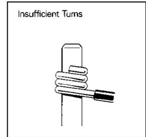
Wire-wrapping is a precision technique. Proper bit and sleeve selection is important. Incorrect choice can lead to problems ranging from pigtails to loose wraps.
