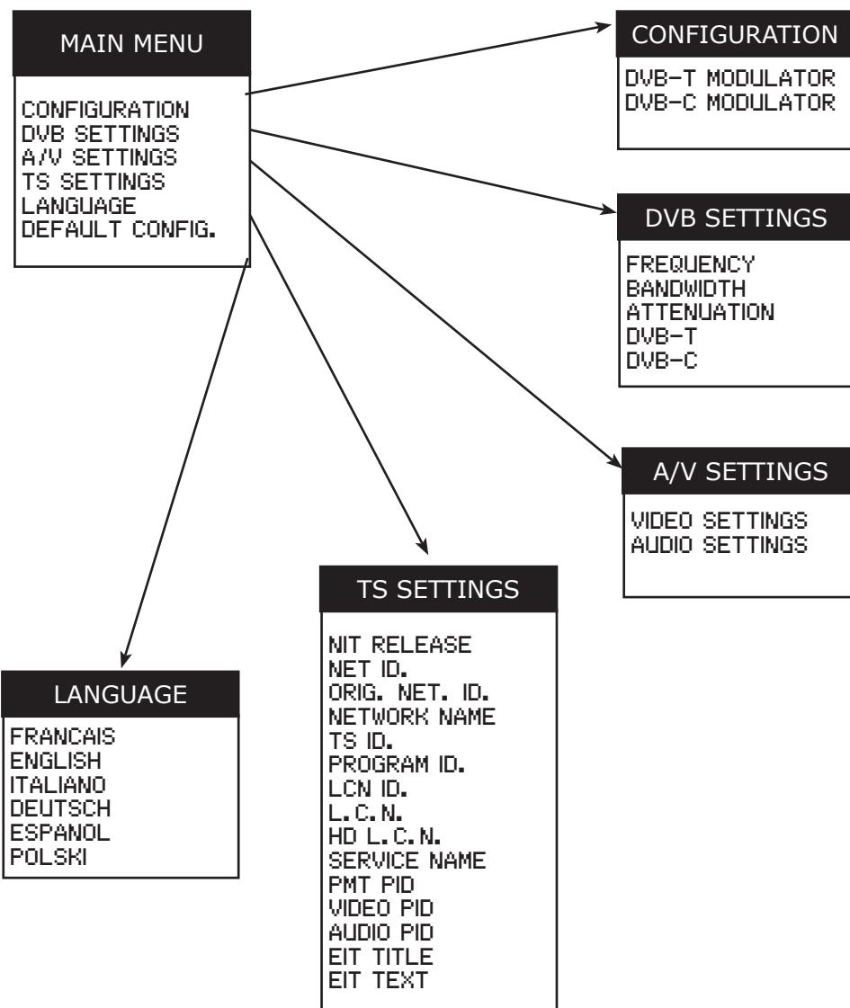
In order to go from one menu to the other use the MOVE **UP/DOWN** keys to select the menu option. Press the **ENTER** button to select this option. Press the **CANCEL** button to go back to the previous menu.
