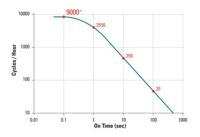
SOLICON Solid State Contactors have advanced switching technology which allows them to operate a motor at a start/stop switching frequency of 9000 cycles/hour\*, switching speed never reached before by a solid state, electromechanical or hybrid contactor.
