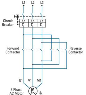
In some cases the direction of the motor (forward/backward) needs to be controlled in such cases 2 contactors need to be used together with an interlock to accidental prevent maneuver.
