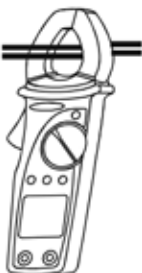
Fig. 6: Use of clamp during DC current measurement.
